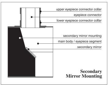
tabs of the mirror holder sit on the eyepiece side of the main body and cover the whole width of the face of the tube. The two foot tabs sit similarly on the opposite face. Push the mirror holder in until it is flush with the end of the main body and secure the tabs with 4 paper clips.
